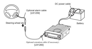
By removing or cutting the cable before turning on will sound alarm. To turn off the alarm, press PWR key to turn off the power. The alarm is canceled and turns on normally when PWR key is pressed next time.
