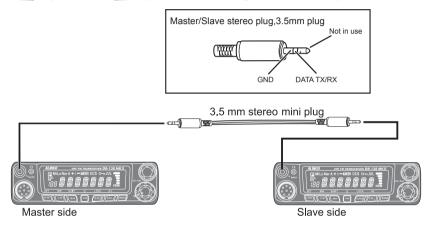
3. Press master unit's [PTT] key, LCD displays "CLONEXX". Slave unit displays "CLONEXXX". When the cloning is successfully finished, the slave unit will restart. Turn off the power, disconnect the cable and repeat step 3 operations to clone the next slave unit.
