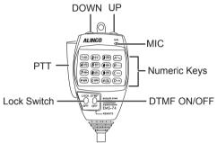
You can operate the transceiver by keypad or input desired frequency or channel through the EMS-74 microphone. Keypad operations may be blocked for dealer-programmed units.
