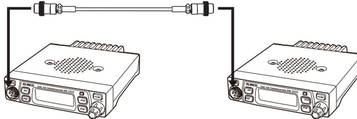
3. Press master unit's [FUNC] key, LCD displays "**CLONEXX**". Slave unit displays "**CLONEXXX**". When the cloning is successfully finished, the slave unit will restart. Turn off the power, disconnect the cable and repeat step 3 operations to clone the next slave unit.
