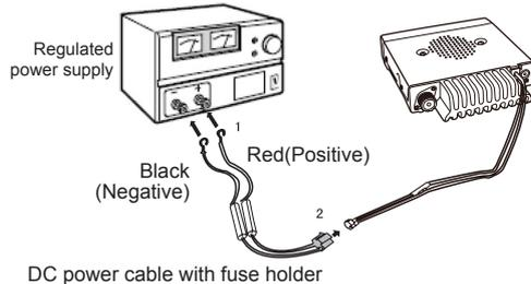
2. Connect the transceiver's DC power connector to the connector on the DC power cable.
