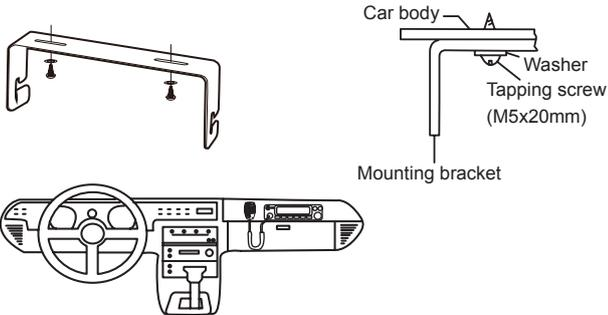
2. Position the transceiver, then insert and tighten the supplied fixing screws.
