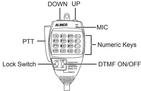
Following operations are available using keypads on the EMS-74 microphone.
